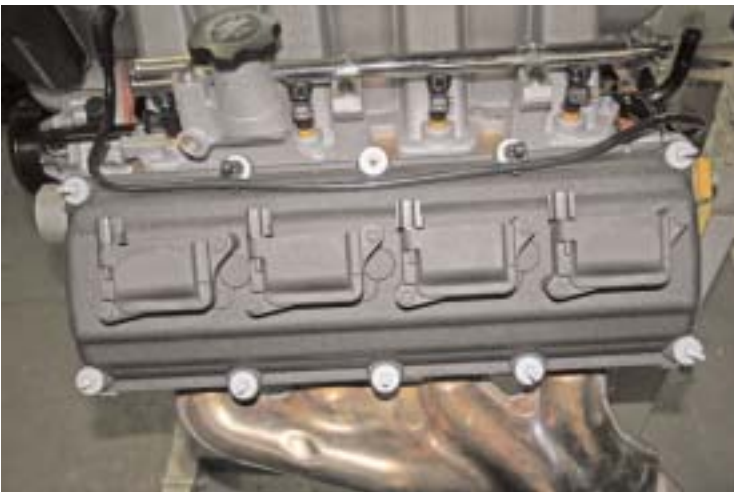
NO Spark Plug Wires!!Coils are right on top of the plugs
