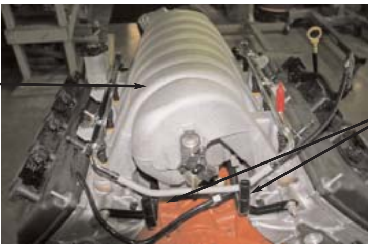
NO Spark Plug Wires!!Coils are right on top of the plugs
