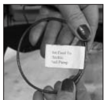
Connect the brown fuel pump wire directly to the fuel pump. Do not connect thru buss or panel.
