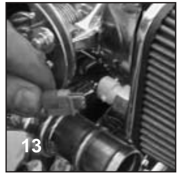
Install air temp sensor at rear of Street & Performance air cleaner
