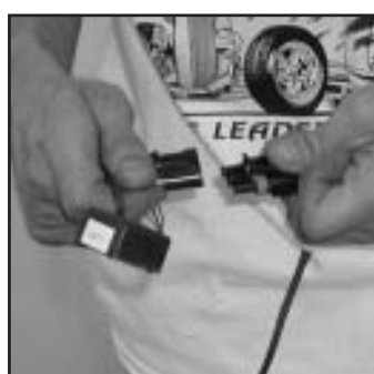
Install Vat by-pass to Vats plug in harness.
