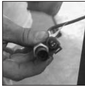
On Vette remove Coolant Temp sensor and replace with IROC/TA. pt#12551708. Part is available from Street & Performance or G.M. The Collant Temp Sensor uses a three prong plug.
