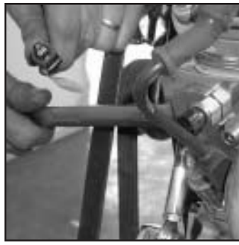
On Vette remove Coolant Temp sensor and replace with IROC/TA. pt#12551708. Part is available from Street & Performance or G.M. The Collant Temp Sensor uses a three prong plug.
