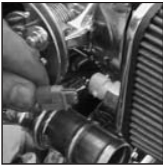
Install air temp sensor at rear of air filter
