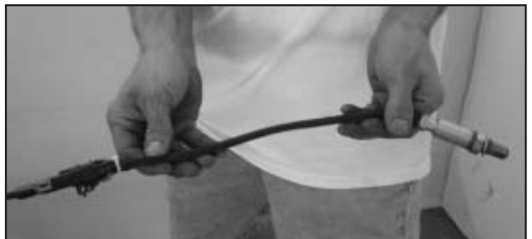
Check the O2 sensor for breaks or chafing. Replace if necessary. Available from G.M or Street & Performance
