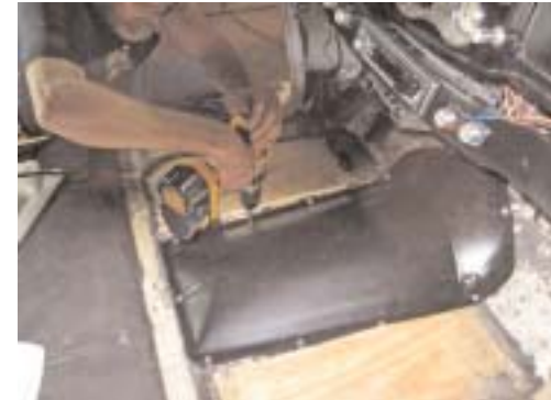
The S&P crew made a new tranny cover and bolted it into place.
