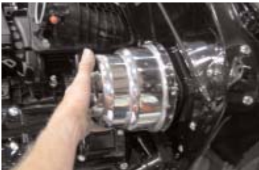
A Rex big brake booster had to be changed to a 7 inch booster to clear the HEMI valve covers.
