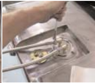
Rex already had a Rock Valley Stainless tank, so we sent it back to Rock Valley to have a high pressure pump installed. The pump will have a feed and return even though the HEMI only uses one fuel line. S&P has a fuel filter regulator which regulates the fuel and sends the extra back to the tank.
