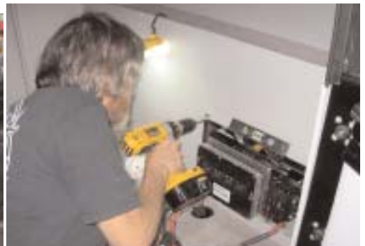
Larry made a bracket to hold the computer, fuse panel and relay in one spot behind the rear seat.
