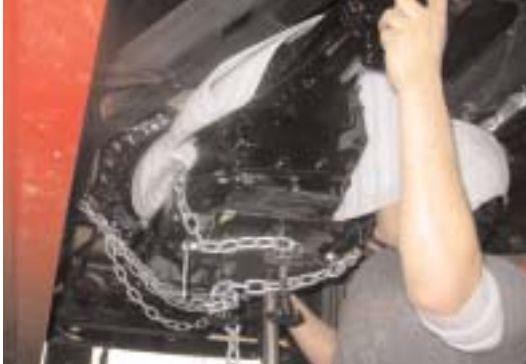
Then the 545RFE Transmission was raised into position and bolted to the HEMI. Knowing that the 545 RFE was bigger than the 350 transmission the tunnel was trimmed out before the final install of the tranny.
