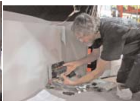
Since the under dash heat and air took so much room, S&P made the harness longer to reach the back seat and the computer was mounted there.
