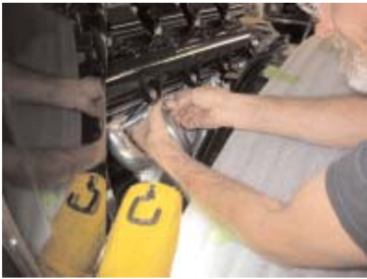
S&P makes a set of block hugger headers for the HEMI that comes with two O-2 sensor buns. The front two O2 sensors will be used to help with fuel mileage and performance.
