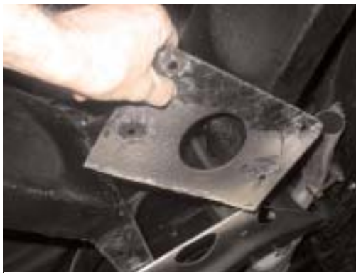
Larry lowered the HEMI into the engine bay with the S&P engine mount adapter plates and bolted them right back to the GM mounts.
