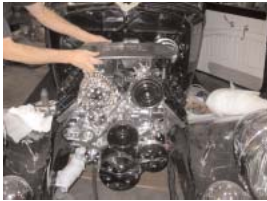
The factory alt and air was used but the power steering pump had to be replaced with a GM pump with an S&P pulley. The Mopar pump puts out too much pressure for the Ford rack on the 34. Also note that a 5.7 HEMI from a car will have 6 groove pulleys and the trucks will have 7 groove pulleys.
