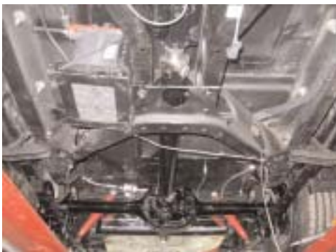
The gears in the 8 inch Ford rear end were changed to 3:73. S&P made and balanced the drive shaft.
