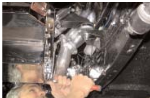
Connecting the exhaust to the collector. Also note the S&P custom short oil pan which allows for more ground clearance. The engine mounts can also be seen clearly.
