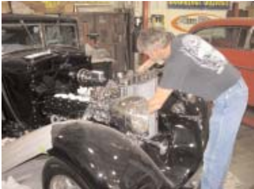
Larry sent off to Griffin the radiator and had them build a radiator to fit the 34 with the proper outlet/inlet for the HEMI.
