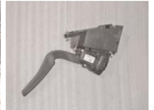
Larry decided to use the 2005 truck gas pedal on this install.
