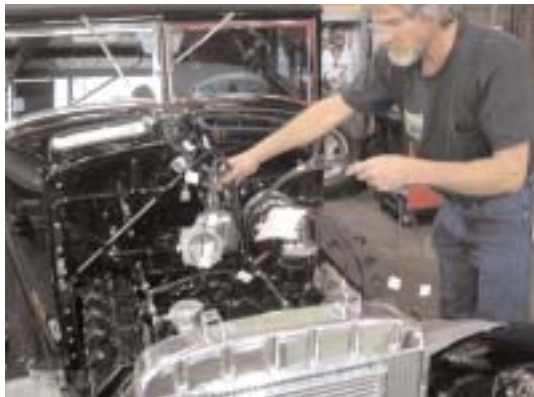
Larry runs the S&P wiring harness from inside the car to the engine compartment
