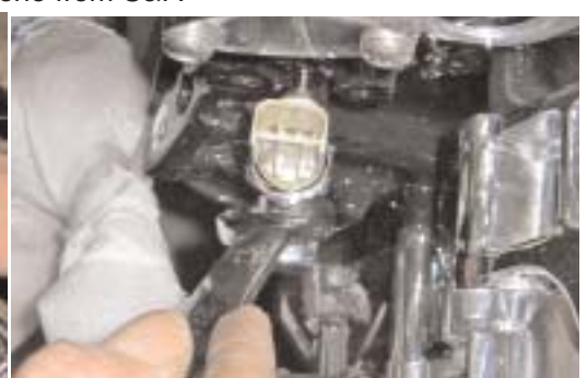
The oil pressure sending unit can be installed in the factory location at the lower front passenger side of the block.
