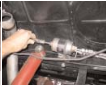
Rex already had a Rock Valley Stainless tank, so we sent it back to Rock Valley to have a high pressure pump installed. The pump will have a feed and return even though the HEMI only uses one fuel line. S&P has a fuel filter regulator which regulates the fuel and sends the extra back to the tank.
