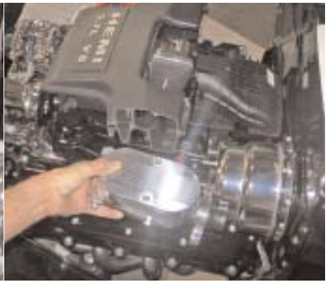
The HEMI air box would not clear the master cylinder on the firewall, so Larry trimmed off part of the air box and will cut a piece to seal up the end of the box.
