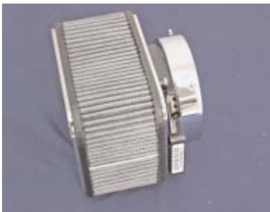
S&P Air Cleaner with built in 5 pin MAF
