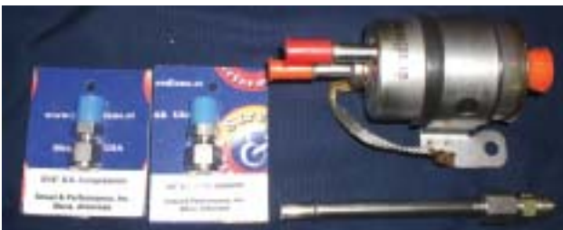
S&P S.S fuel filter kit which has the regulator built into the filter. This filter also has a single line to the engine and a return line to the tank. Kit come with AN6 adaptors and quick disconnect for AN6 adaptor. These parts can also be purchased serarately. S&P also provides a Areo-Quip single-braided fuel line kit from the engine to the frame.
