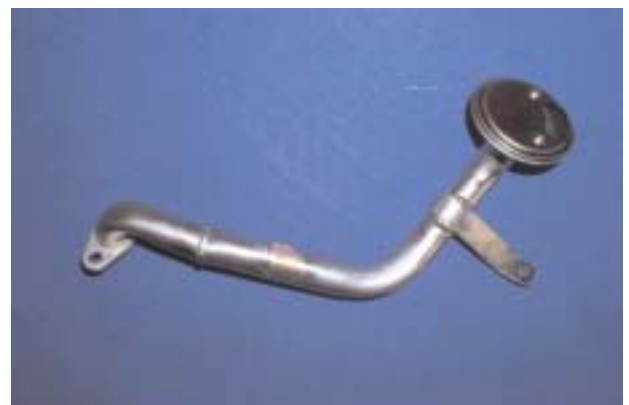
Charlie's Oil Pans located in Norton, Ohio, who provided us with this mid sump aluminum oil pan. When you change the pan to a mid sump, you must also have the oil pick-up tube modified.
