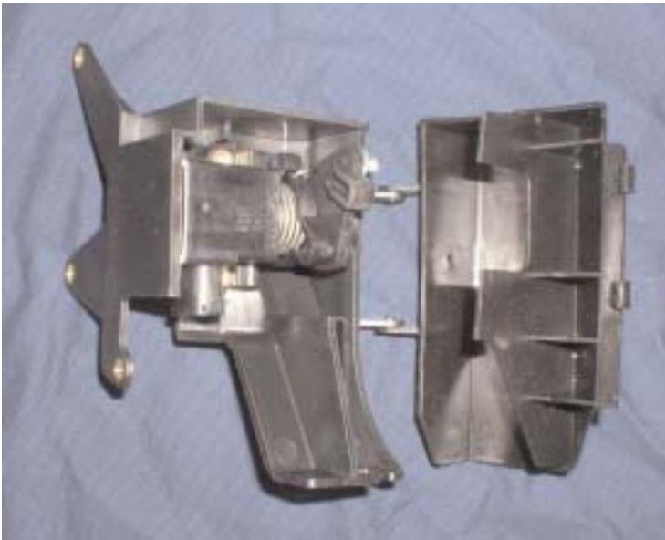
The drive by wire throttle activator box can be mounted almost anywhere under the dash or in the engine compartment.
