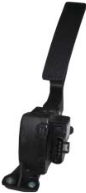
2004 design pedal with activator assembly. can be mounted to the firewall in some applications . This type pedal does not require a throttle cable because the wiring harness plugs into the pedal assembly.
