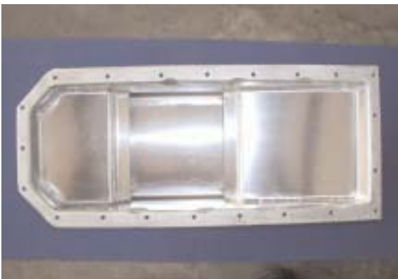
Charlie's Oil Pans located in Norton, Ohio, who provided us with this mid sump aluminum oil pan. When you change the pan to a mid sump, you must also have the oil pick-up tube modified.
