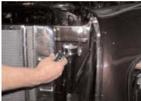
34 The hose from the bottom of the reservoir back to the pump should be #8 or 5/8" hose and be rated for 20" to 27" of vacuum. If not rated for sufficient vacuum the hose may collapse & starve pump fluid flow.
