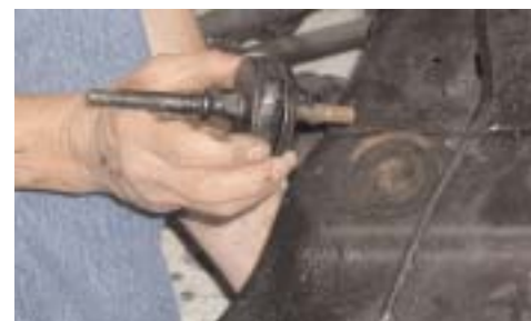
7 Tom removes the old front motor mounts in preparation for the new side mounts which will reduce engine vibration. The original motor mounts interfere with new style power steering pumps.
