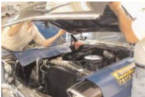
2 Off with the Hood. After carefully marking the hinge locations to aid us during reinstallation, the hood is carefully removed.
