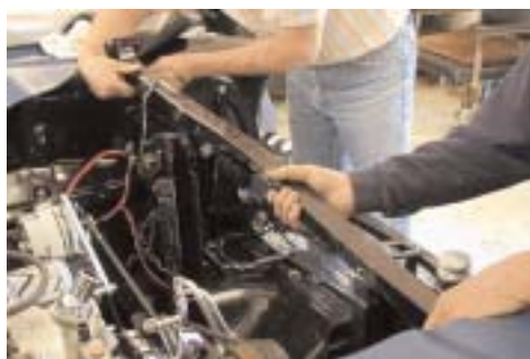
3 Tom and Archie removed all of the front radiator housing and support framework. Bolts are hidden in a number of locations, including underneath the frame pan, so be patient.
