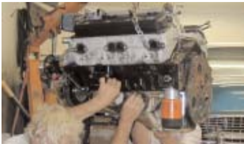
14 Most LT-1 engines use an oil cooler which we removed because the engine oil cooler is not needed in the 55-57, where the Vette or IROC engine set half way under the cowl & the hood set on top of motor holding lots of heat in engine compartment
