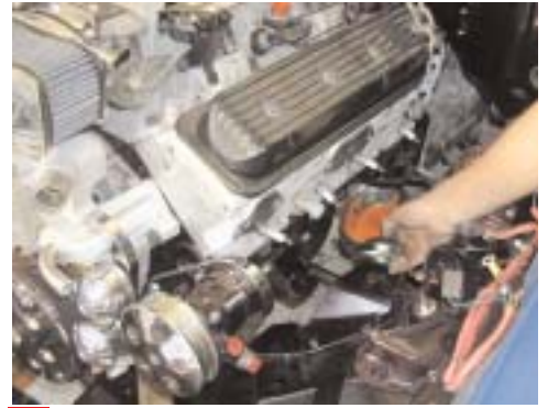
18 The remainder of the motor mount kit is installed during installation of the motor.
