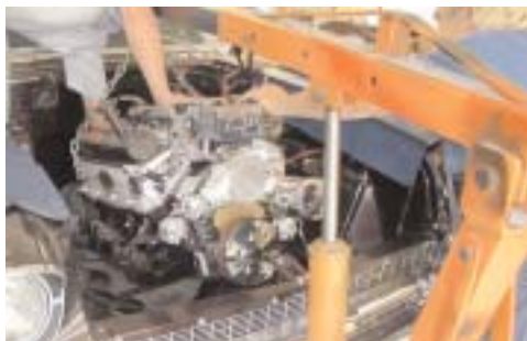
17 The LT-1 Factory Bracket Kit did not work in the 55-57 installation so we picked Street & Performance alt, air, power steering kit in chrome. The reason we went to chrome was for the easy maintenance and good looks. We used the wide style brackets (Vette Style) because we moved the battery to the back, on 57 if the battery box is in stock location you would have to run Street Rod Style brackets. On 55-56 you can run either because the battery is is on the firewall
