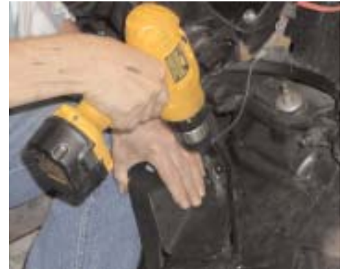
8 With the Side Motor Mount Kit from Street & Performance, it bolts in, no welding is necessary. The new side motor mounts are positioned, drilled and tapped, directly through the frame cross member.
