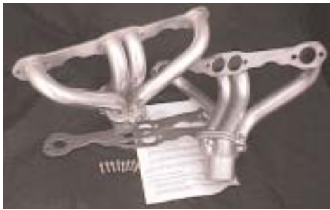
55-57 Chevy small block Pro Car headers from Street & Performance with all stainless head flanges and collector flanges and O2 buns installed.
