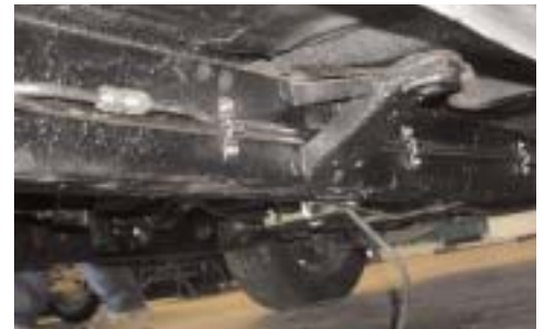
37 Hard line stainless steel fuel lines by James Miller of Tube Tech. Both lines are stainless steel. Avoid rubber fuel lines.
