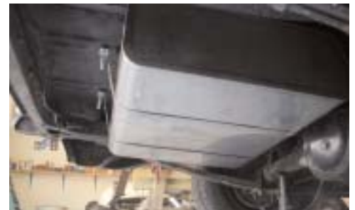
38 The addition of a stainless steel gas tank from Rock Valley added more fuel capacity and had the high pressure fuel pump already installed in the tank. The larger size fuel tank required removal of the spare tire mounting hole. The Rock Valley tank was complete with stainless steel mounting straps. The pump in the tank is the most desirable method because it is a pusher, reducing the opportunity for vapor lock in hot weather. Internal pumps are quieter and run cooler. If you decide for an external pump planning pump location is very important in maintaining fuel flow.
