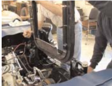
4 After removing the radiator and radiator frame assembly you can prepare your surfaces depending upon your application.
