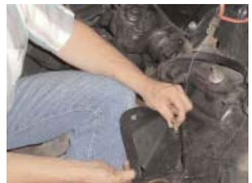
9 The new mounts are bolted into place. By locating motor mounts & power steering first, we can clean, paint & detail the entire engine compartment
