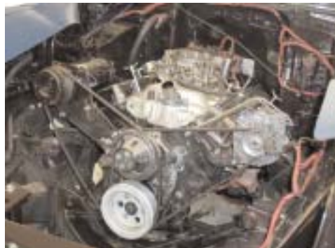
5 The old 350 stands ready for removal
