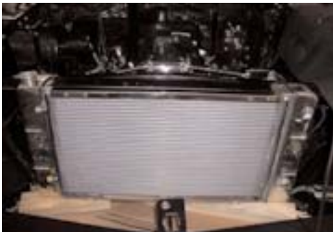
32 With the radiator in place, Tom is able to install the Goodyear radiator hoses that were purchase from S&P with the cross flow radiator.
