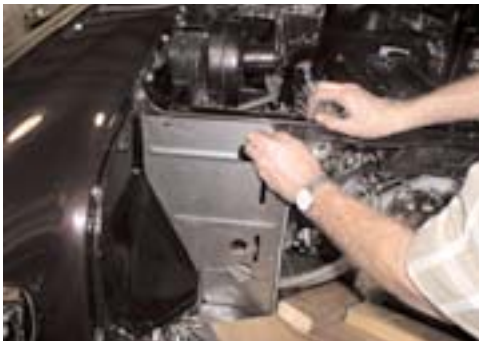
30 Tom checks the fit of the side panels before painting them to match the cars black cherry finish.
