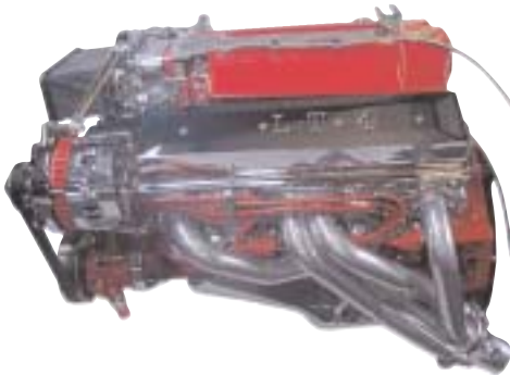
55-57 Type III headers for rack and pinion type steering. Comes with collectors and O2 buns installed.
