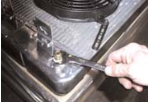
31 S&P provides an adjustable thermostat switch that has a fitting and sensor that can be placed into the port which is added to the S&P cross flow just for this purpose.
