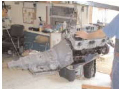
16 The new engine and transmission are now ready to install.
