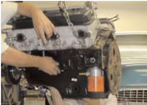
13 The LT-1 engine is detailed. On Vette engines the oil pan has to be changed to IROC oil pan to clear the 55-57 front cross member. All IROC/TA, SS Impala, Cad & Buick oil pan will clear front cross member with out any modifications
