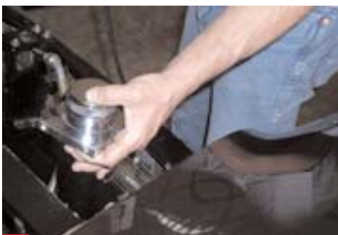
33 With the side panels painted and bolted into place, Tom mounts the radiator over flow reservoir to the passenger side panel
