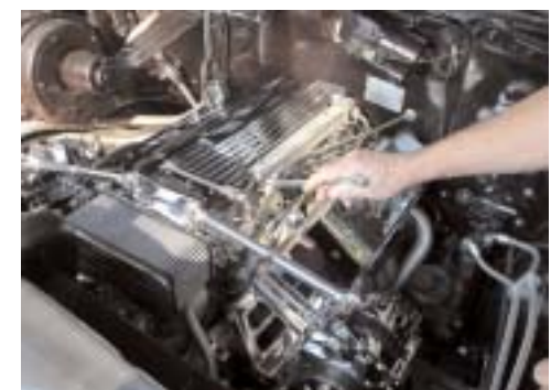
39 Tom is installing the Lokar LT-1 Braided throttle cable. The LT-1's w/4L60E transmission do not run detent cables like 93 & earlier.
