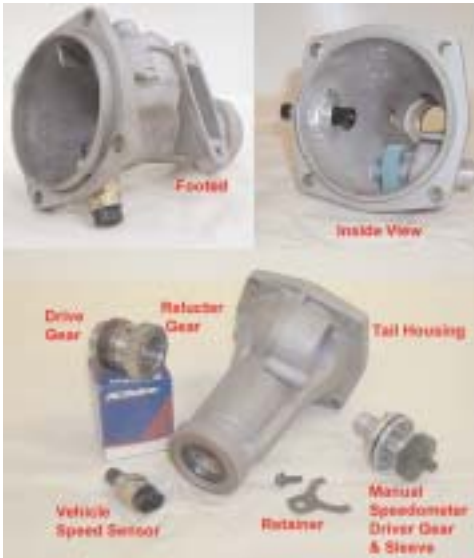
The Tail Housing Kit from Street & Performance lets you add manual speedometer to your 4L60E transmission. You need to know your gear ratio & tire roll out dimension.
