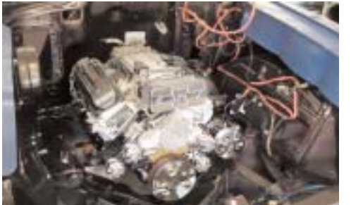
19 With the LT-1 sitting in position we can now build the rear transmission mount.
