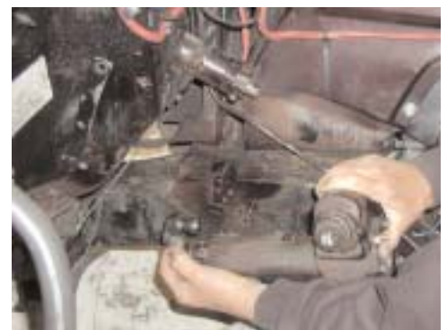
10 Off with the old 57 steering gear box. The new power steering is the 605 55-57 Gear Box Kit from Mullin Steering Gear or your local hot rod shop.
