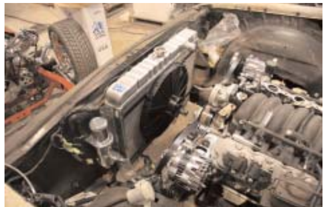
The Griffin radiator came with a Spal fan already mounted and the 1 1/4" inlet on top and a 1 1/2" return on the bottom passenger side for the LS-1 engine.
