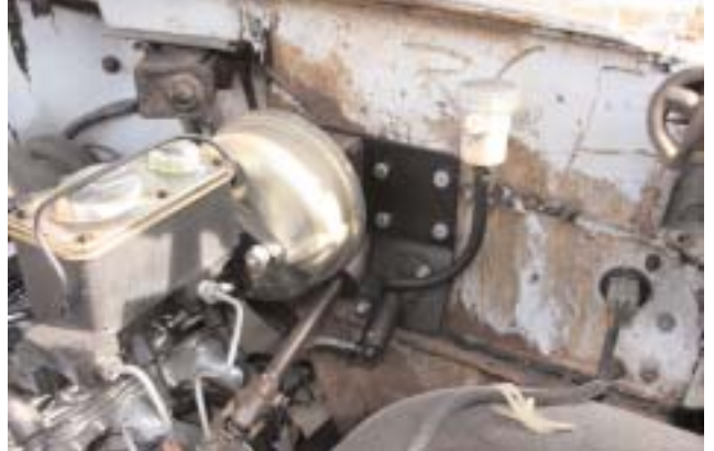
With the bracket and brake booster mounted we then installed the slave cylinder reservoir to the fire wall.
