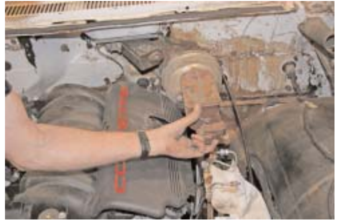
A small brake booster will clear the coils and valve cover but we will need to modify the valve cover vent to allow the engine to breathe.
