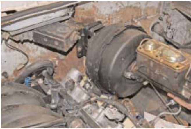
Above shows that a large power brake booster will hit the coils and valve cover.
