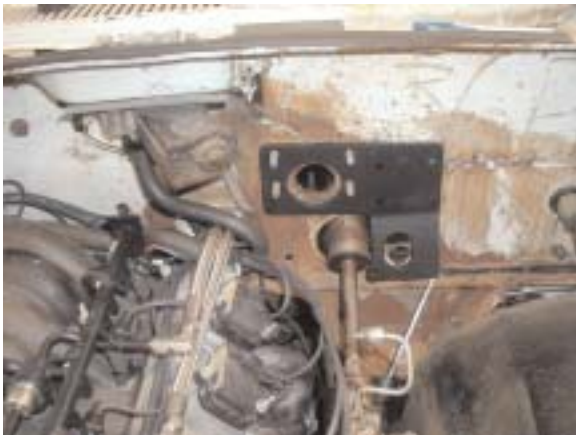
S&P custom made this mounting bracket for the clutch slave cylinder. This bracket mounts behind the brake booster. S&P offers this bracket for a variety of applications.
