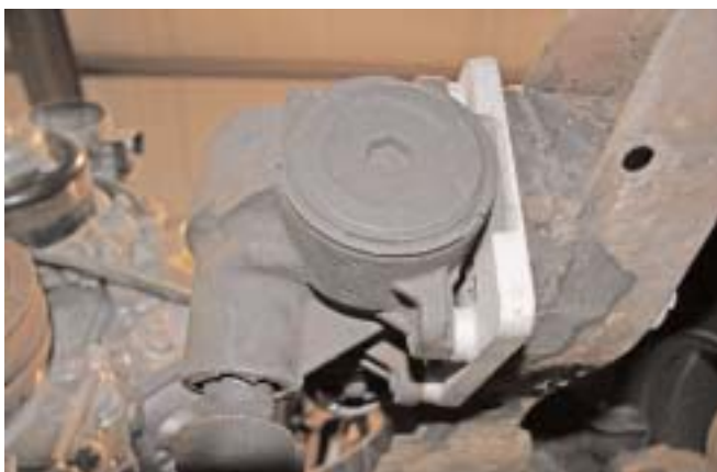
An aftermarket adapter plate allowed the mounting of a 605 gear box.
