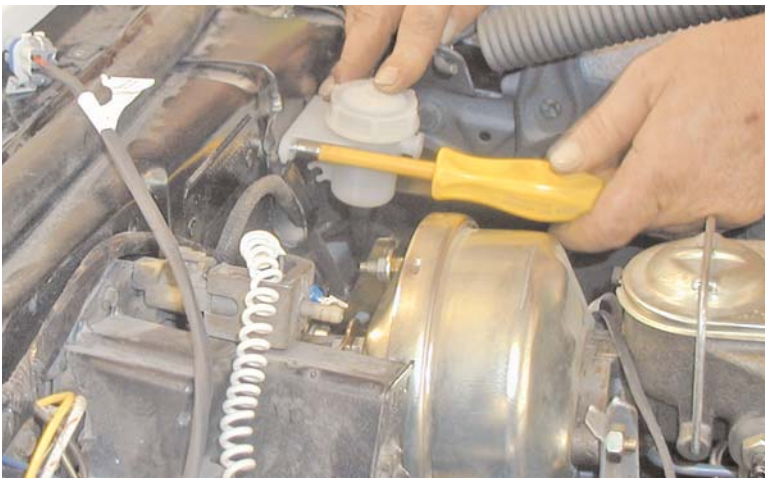
Mounting the 6 speeds hydraulic clutch cylinder reservoir to the firewall to ease the checking of fluid level.
