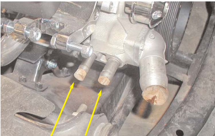
The small fitting closest to the firewall goes to the heater and the larger fitting closest to the waterneck is the return from the heater.
