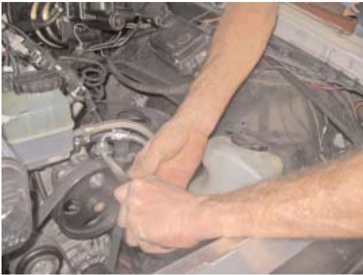
GM pump uses a 16mm o-ring on the pressure side.
