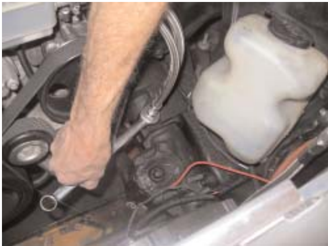
Larry makes up some S&P braided lines for the power steering. The gear box uses 18mm o-ring & 16mm o-ring to AN6.
