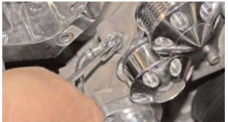
Lokar cables were used to hook up the throttle and cruise.
