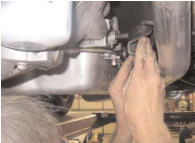
Original floor shifter cable bracket is bolted to the 4L60E trans.
