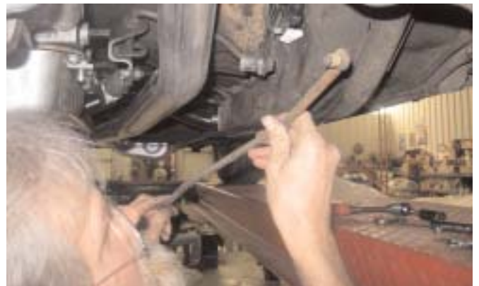
Original floor shifter cable bracket is bolted to the 4L60E trans.
