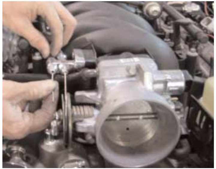
Lokar cables were used to hook up the throttle and cruise.
