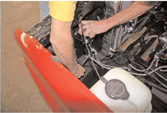
The S&P power steering hose kit is then connected to the S&P remote reservoir mounted on the radiator support.
