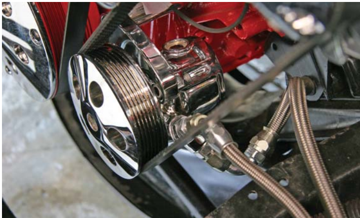
The S&P chrome power steering pump is mounted low on the driver side and cleared the frame rail without problems. Custom power steering hoses provided by S&P are then installed.
