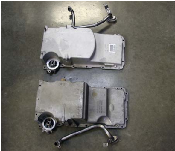
Vette LS-2 pan shown above has to be changed to a 98-02 Camaro pan to clear the cross member. Truck pan can be used if the vehicle does not set to low.
