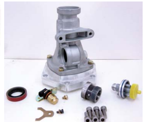
96-Up 4L60E 6 Bolt to 4 Bolt Tail Housing Adapter. Comes with tail housing gears and hardware For Manual Speedometer. Gear ratio and tire rollout is needed when ordering.
