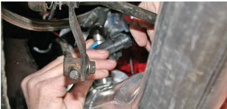
While under the truck we plugged the wiring harness into the Oxygen sensors located in the header collectors. Then the gear selector linkage was attached.
