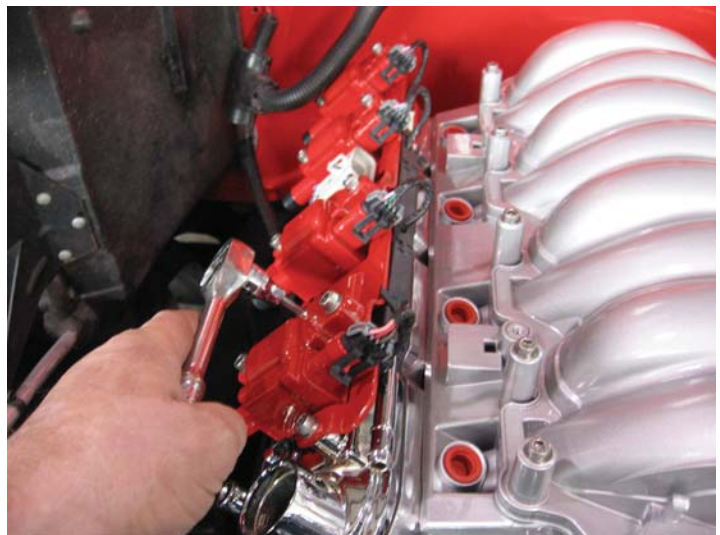
We painted the coils and chromed the coil rack which makes for easier cleaning. Tighten the ignition coil mounting bolts to 12 N·m (106 lb in).
