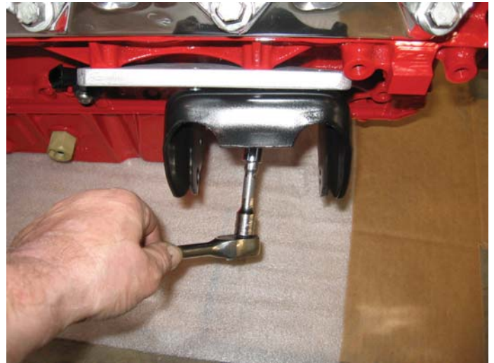
The factory mounts are then bolted to the S&P adapter plates. S&P recommends the use of anti-seize compound on all bolt threads.
