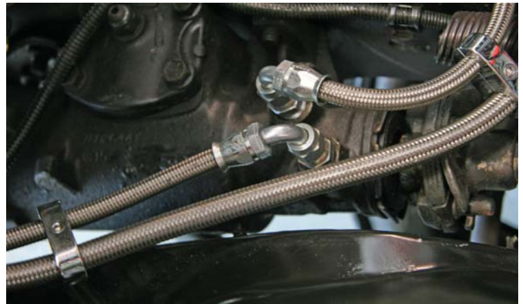
The pickups steering box uses an 18mm o-ring & a 16mm o-ring to AN6 adapters to connect to the S&P hose kit. After making the connections fill the remote reservoir with GM 12345867 Power Steering Fluid or Valvoline Pyroil Power Steering Fluid PSC-12.
