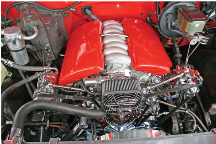
S&P built the MASS AIR FLOW into the air cleaner and S&P smooth top covers were painted as well as the plastic intake. The top covers are available in black, white, red and carbon fiber.
