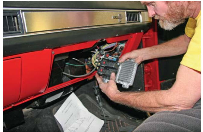
The reprogrammed computer is mounted behind the glove box and the ALDL connector is mounted under the dash for easy access. The New Street & Performance Performance Plus Tuner/Scanner/Programmer. The performance plus will allow you to alter the computer programming such as gear, and tire diameter changes, engine tuning, shift points, etc. It also scans for error codes.
