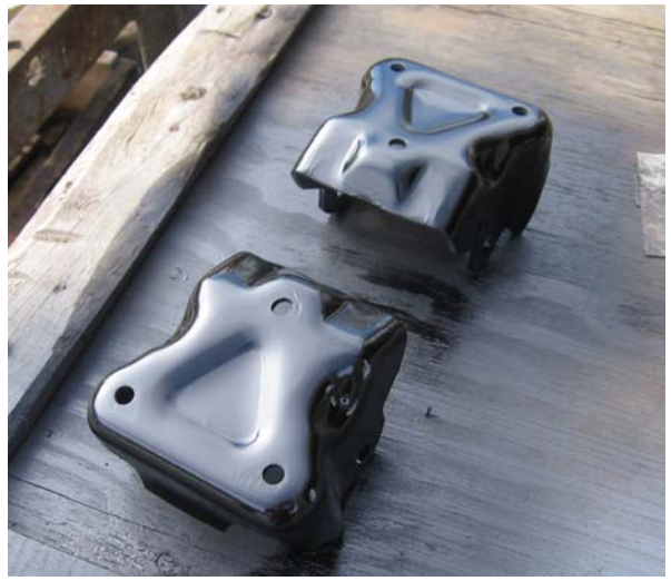
The late type vehicles use clam shell mounts, Sometimes these clam shells will have a knot on the back that will have to be ground flush to the back of the mount.
