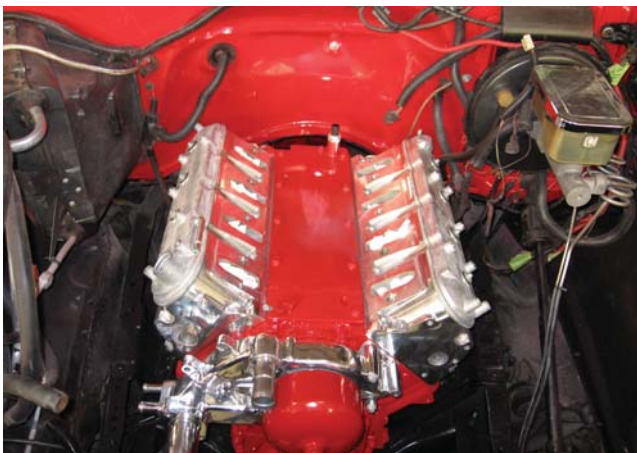
With the engine in place, it is best to leave the front mounts and stands loose until you get the rear cross member bolted in. Once all the bolts are in place then tighten them down.
