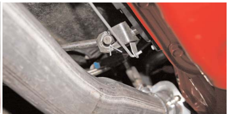
While under the truck we plugged the wiring harness into the Oxygen sensors located in the header collectors. Then the gear selector linkage was attached.
