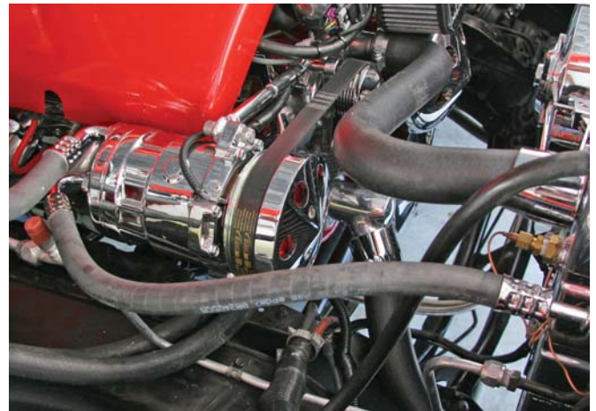
All of the AC lines were done with O-ring fittings to prevent leaks, then S&P's chrome shop chromed the fittings right on the hose.
