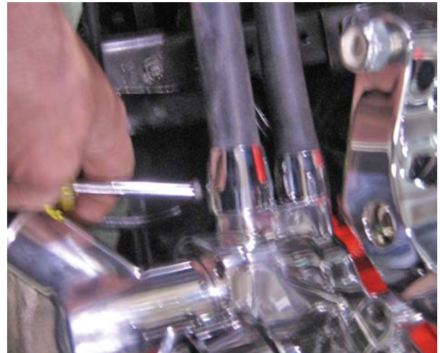
The heater hoses were hooked up to the water pump fittings. The 5/8 bib is out to the heater and the 3/4 bib is the return. We also install S&P hose clamp covers to clean up the connection.
