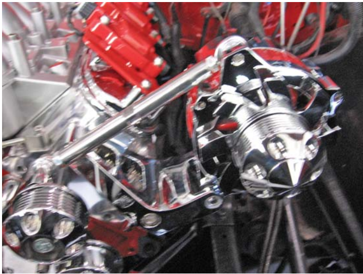
A CS-130 140 amp Alternator was used. This alternator has a small size and can be built at S&P to an output of 140 amps.
