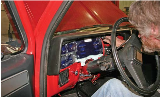
Larry installs the Dakota instrument cluster into the dash. Since Dale chose to use the electronic speedometer, he did not need to change the tail housing on the transmission. If you elect to retain the original manual speedometer you will need the tail housing adapter below.
