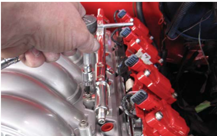
Install the intake manifold bolts and fuel rail stop bracket
