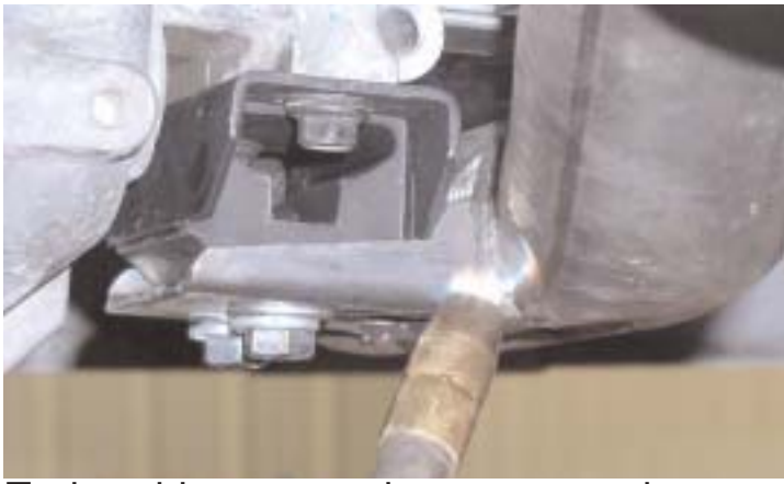
Tack weld mount to the cross member.
