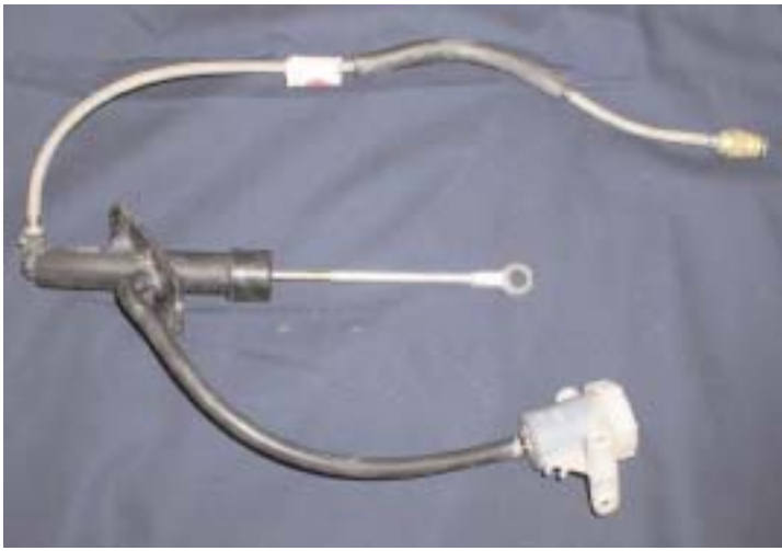
Left, shows the hydraulic clutch cylinder assembly, needed to operate the T-56 Clutch. GM Part #12570277
