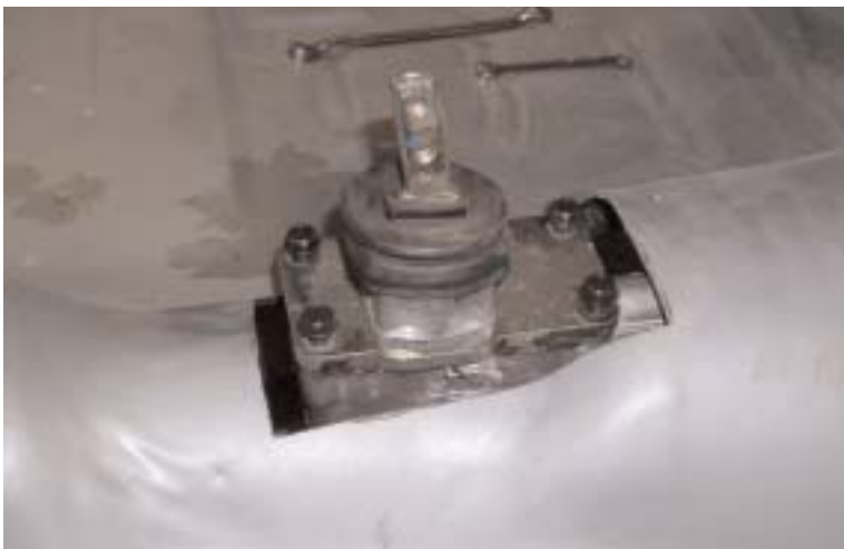
This photo shows the factory shifter in place. While this shifter is a good shifter, we wanted to replace it with the B&M Short Throw Sport Shifter Part # 45052 for a 93 - 2003 T-56 Transmission. Remove the 4 bolts holding the factory shifter in place and pry up on the shifter base plate.
