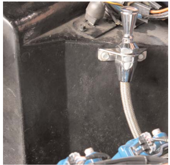
Left we install Lokar's ED-5008 Engine dipstick chromed by S&P. Right the Lokar firewall mount trans dipstick TD-34L60EFM also chromed by S&P
