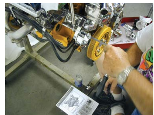
Install the passenger side idler bracket with the two 3/8 x 4 provided with the idler bracket kit
