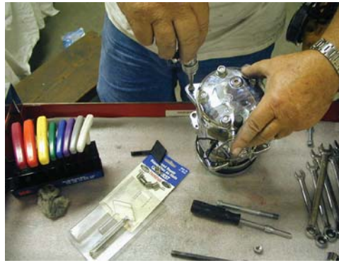
When using valve covers other than stock, bottom back ear on A/C Compressor must be heli-coiled for 3/8-16 threads. (Shown tapping lower ear at rear of compressor)
