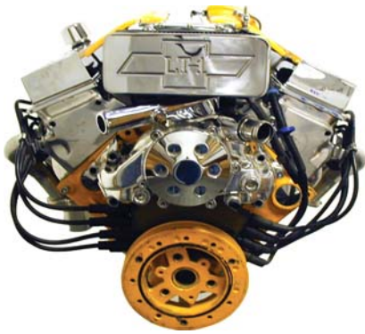
96 LT1 Camaro Motor with block ground smooth with polished heads and water pump. matching chrome valve covers, aluminum dress up plate and plastic Corvette top covers
