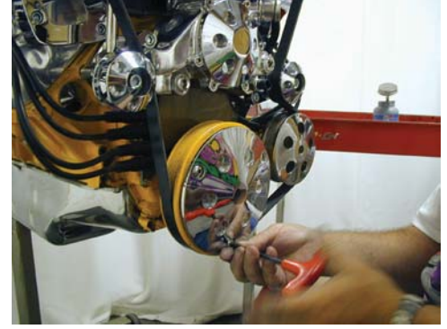
Installing S&P LT1 Crank Cover with 3/8 bolt provided (93-97 Camaro, Trans-Am and SS Crank pulleys use one cover and Corvette use a 92-96 use a different cover. LT4 uses a Special cover for it balancer)
