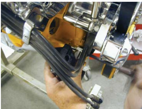
Remove the two lower spark plug wires from the distributor for the mounting of the coil bracket.
