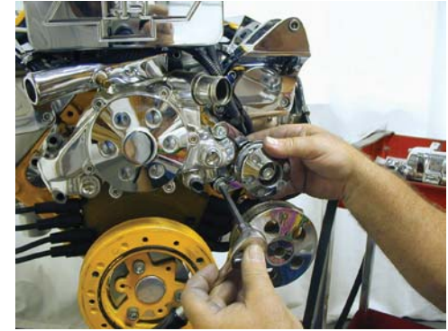
Tighten the Idler Bolts
