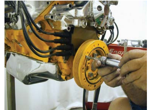
For installing the crank cover, you must tap three of the holes in the balancer with a 3/8-16 tap. Hold the cover up to the balancer to locate which of the three holes need to be tapped. Holes DO NOT have to be drilled for tapping.
