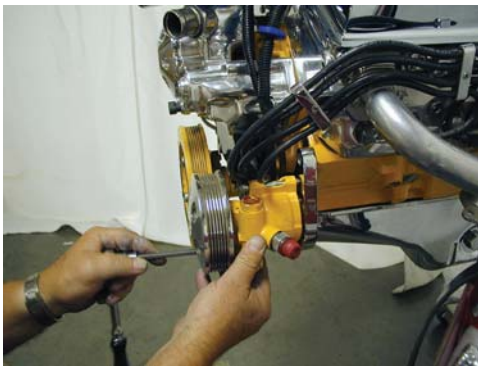
S&P LT1 Power Steering Pump Bracket has a multiple bolt pattern so that the pump can be clocked for better positioning of the pump fitting per your application. Rotate the pulley to allow access to the two 5/16 bolts that thru the pump into the mounting bracket.
