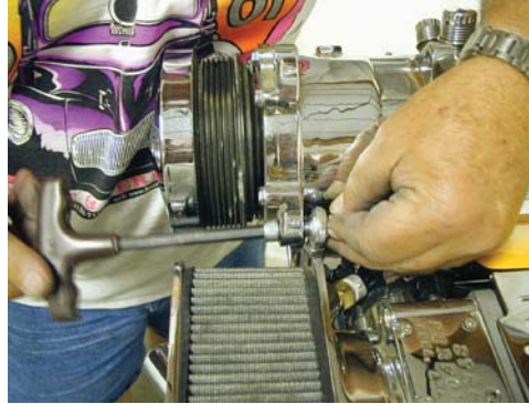
Using 3/8 x 1 3/4 Allen bolt with 3/16 spacer and self locking nut provided with bar kit, attach A/C adjusting bar to the ear on the compressor closest to the air cleaner.
