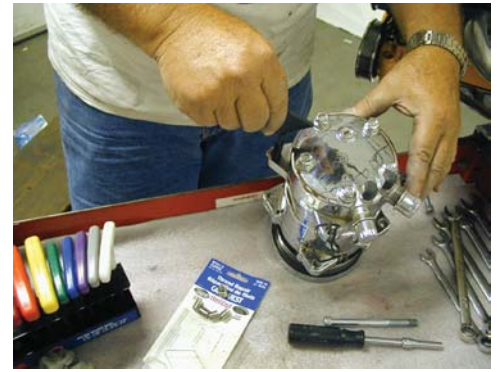
Showing the installation of the heli-coil
