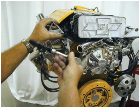
Mounting passenger side LT1 Street Rod Style air bracket with three 3/8 mounting bolt provided.
