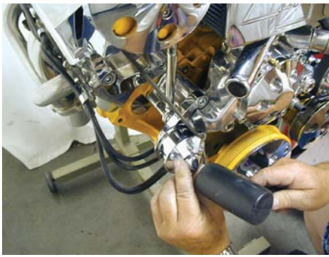
Installing Idler Buttons, Apply lubricant to O-Ring on button and tap into pulley with a rubber mallet.
