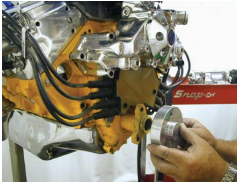
Street and Performance brackets are designed to work with 96 LT4, or 92-96 Corvette balancer. Since our engine is a 96 Camaro Engine Street and Performance provided us with an aluminum crank hub spacer with bolts for spacing Camaro and Trans-Am balancer out to line up like a Vette. On SS impala, Cad, Buick, which are, cast Iron Heads, Crank hub needs to be replaced with a Vette or IROC hub available from GM or Street and Performance, PN 12555283.
