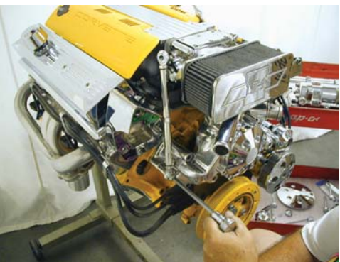
Installing the 7 1/2" s.s air adjusting bar using the 3/8 x 3 1/2 bolt with 1" s.s spacer provided with the alt and air bar kit. (NOTE must be installed before the passenger side idler bracket.)
