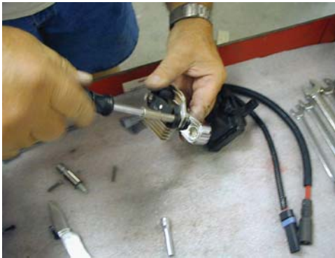
Mounting LT1 coil module on to S&P coil mounting bracket kit with bolt provided with kit.
