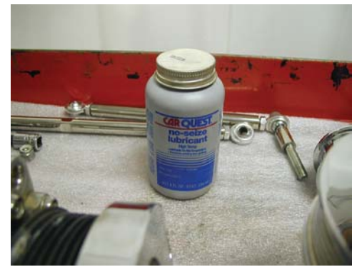
Use Hi Temp Permatex No Seize Lubricant on all bolts where two different types of metal come in contact
