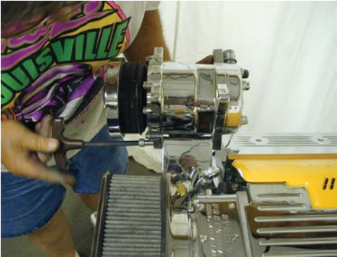
Installing 3/8 x 5" mounting bolt. When not using tall valve covers, a self-locking nut provided with bracket can be used without installing a heli-coil.
