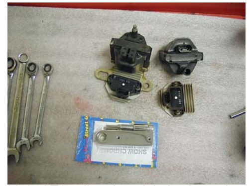
92-95 LT1 coil and module is pictured on left and 96-97 LT1 coil and module is pictured on the right. S&P LT1 Coil mounting bracket is pictured below coils.
