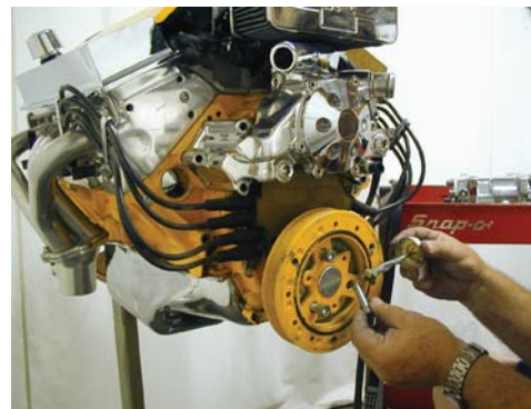
Using anit- seize, install balancer on top of aluminum crank spacer.
