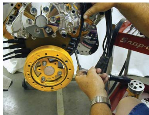
Install the Power Steering Pump Bracket using three 3/8-16 bolts into the two vertical bolt holes to the drivers side of the balancer and the upper side of block.
