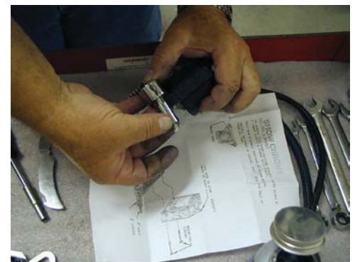
Use 3/8 mounting bolt and 1" s.s spacer provided with kit. Mount to the upper bolt hole to the left of the balancer.
