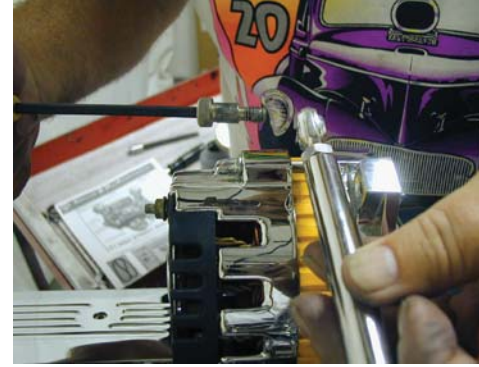
Installing 5/16 s.s. shoulder bolt thru heim into top ear of alternator
