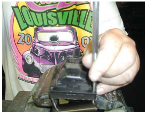
Mounting LT1 coil must grind off head of rivets holding coil to stock bracket then with a punch, punch the rivet out of the coil.
