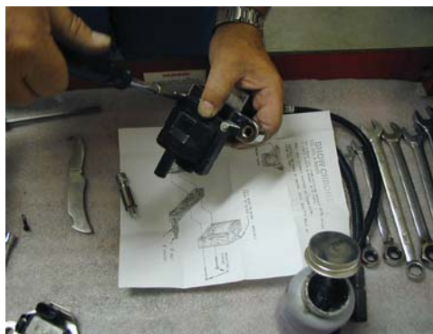
Mounting the LT1 coil to back side of the S&P coil mounting bracket kit as per instruction sheet.
