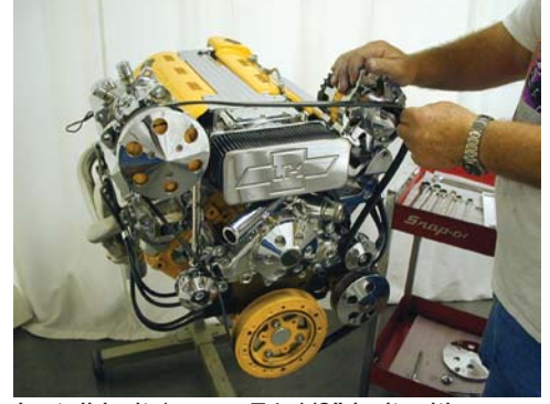
Install belt (use a 74 1/8" belt with Power Steering or a 69 1/4" belt without Power Steering)
