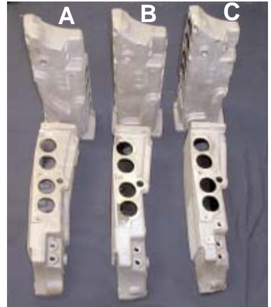
(A) 85-88 plenum (B) 89 Only plenum (C) 90-UP plenum
