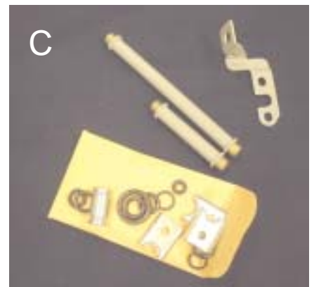
(A) Passenger side TPI tube, 85-92 Vette/IROC T/A are all the same. (B) 85-88 driver side IROC/ T/A, Vette with ninth injector port TPI tube. (C) 89-92 Camaro and 89-91 Vette driver side TPI tube
