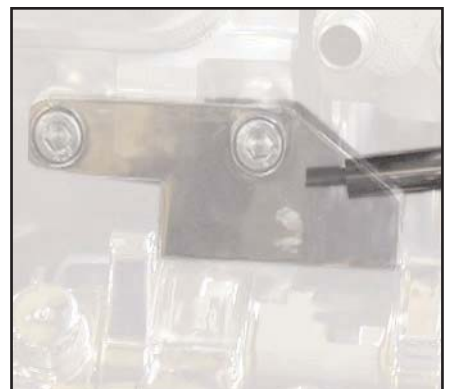
Note Stainless Steel Spacers behind the idler bracket, locate behind the compressor bracket, and screw into the timing chain cover.
