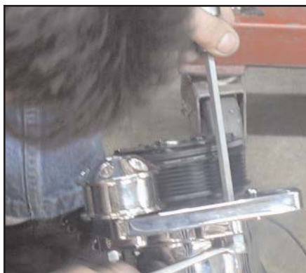
3/8-16 x 1 1/2" Bolt w/ Lock Nut thru Idler Bracket and Air Compressor
