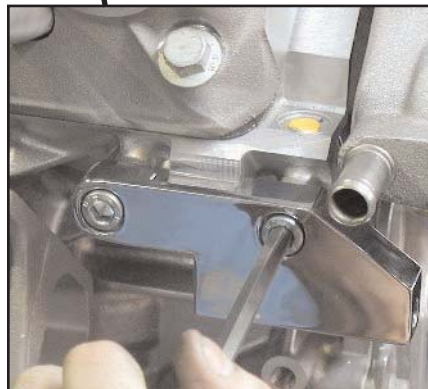
10mm x 25 Bolts thru Bracket into Block
