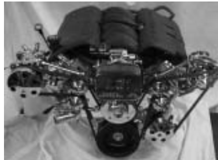
50's & Later High Driver side Alternator High Passenger side A/C Low Driver side P/S
