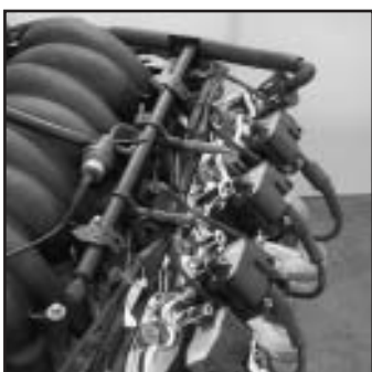
Attached tied wires to the top cover clip bar
