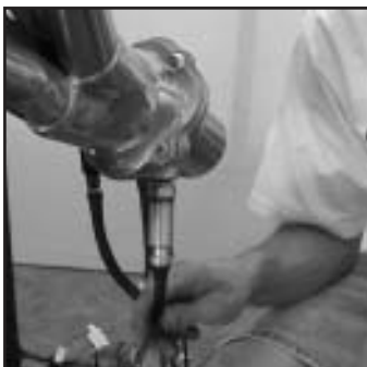
Install the O2 sensor into the front O2 bun on your header collector.
