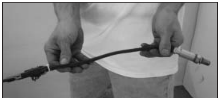
Check the O2 sensor for breaks or chafing. Replace if necessary. Available from G.M or Street & Performance, part #25312202 A/C Delco AF 3-108
