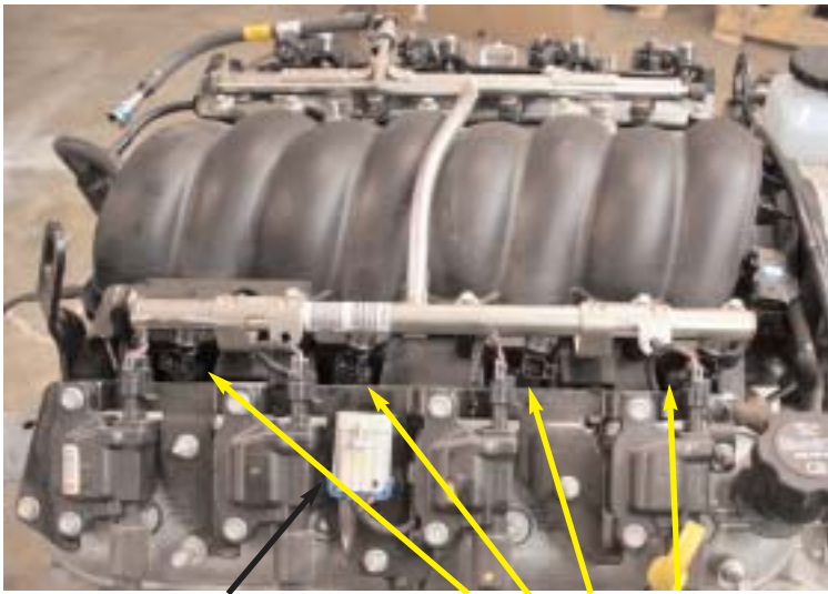
Passenger side master coil plug Injector plug location both sides
