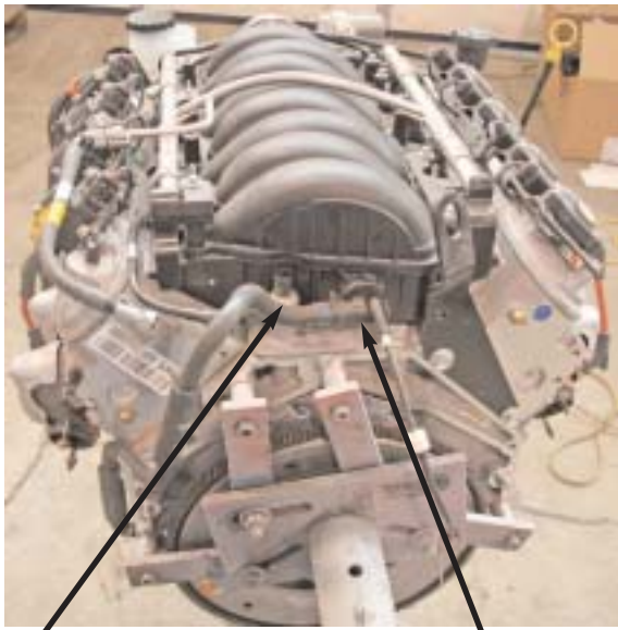
Stock oil pressure sensor Large vacuum port for power brakes and small port for accessories
