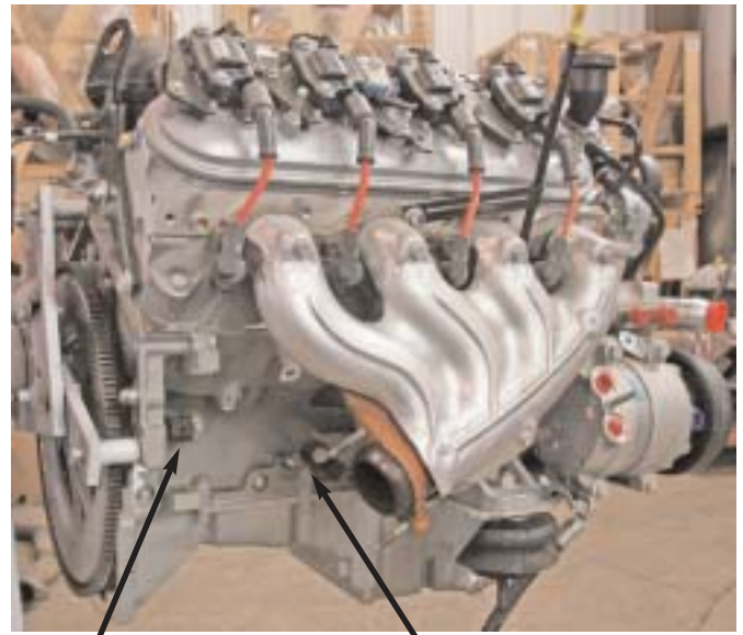
Crank sensor behind starter Passenger side knock sensor
