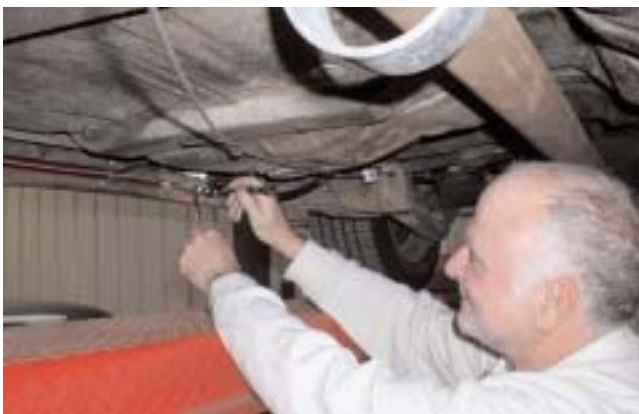
Dominick connects the nylon fuel line from the tank to the stainless hard line mounted to the frame forward of the differential. There are two fuel lines needed, one feed line and one return line.
