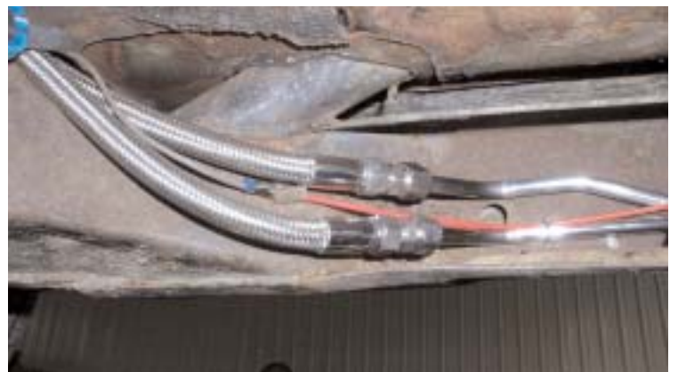
At the forward end of the hard lines, the braided hose rear exit fuel line kit is attached. When making the connection on the fuel line, be sure to coat the threads of the fittings with oil to insure proper seal.
