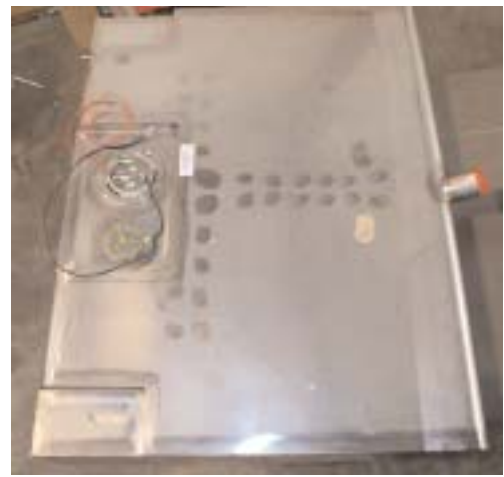
Rock Valley supplied us with a stainless replacement tank with a LS1 fuel pump and replacement sending unit already installed. We added extension wires to the pump and sensor to make the connections to the wiring harness easier after the tank is raised into position.
