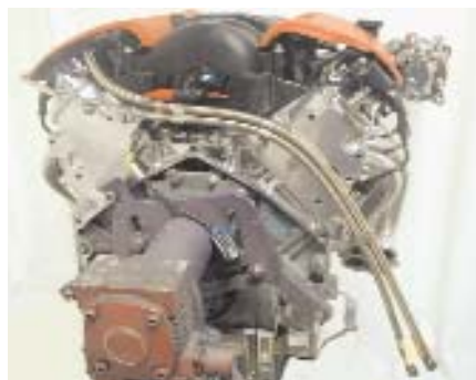
All Passenger Side and Driver Side Fuel Line Kits inc. all connectors, aeroquip braided fuel line, AN6 ends and sufficient length to frame
