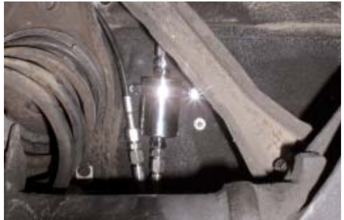
To filter the fuel a S&P stainless fuel filter kit was used. This kit uses a AC DELCO GF481 filter which provides the flow rates needed for injection systems and comes with a mounting bracket and two 16mm to AN6 fittings.
