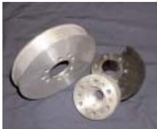
Crank pulley and blower hub adaptor for 6 bolt with male register crank hub.
