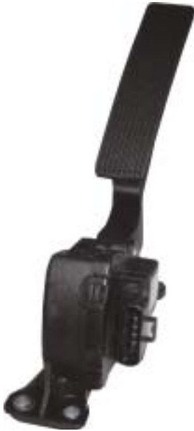
2005 design pedal with activator assembly. can be mounted to the firewall in some applications . This type pedal does not require a throttle cable because the wiring harness plugs into the pedal assembly.
